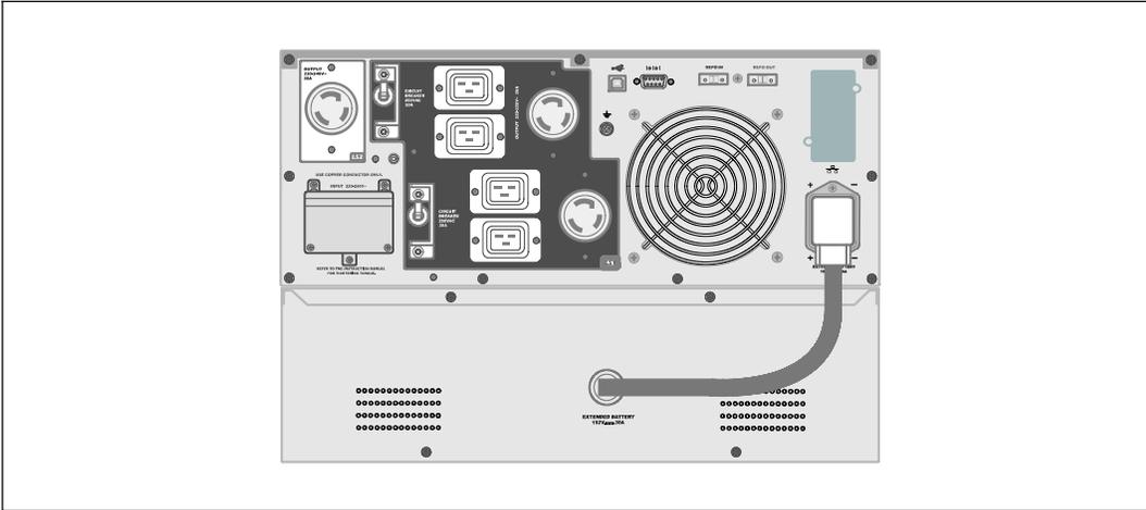
**7** Plug the EBM cable into the UPS battery connector.
